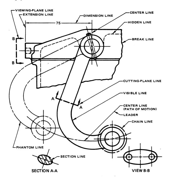
**Fig. 4-1** Application of lines. Reprinted from ASME Y14.2-1992 (R1998), by permission of The American Society of Mechanical Engineers. All rights reserved.
