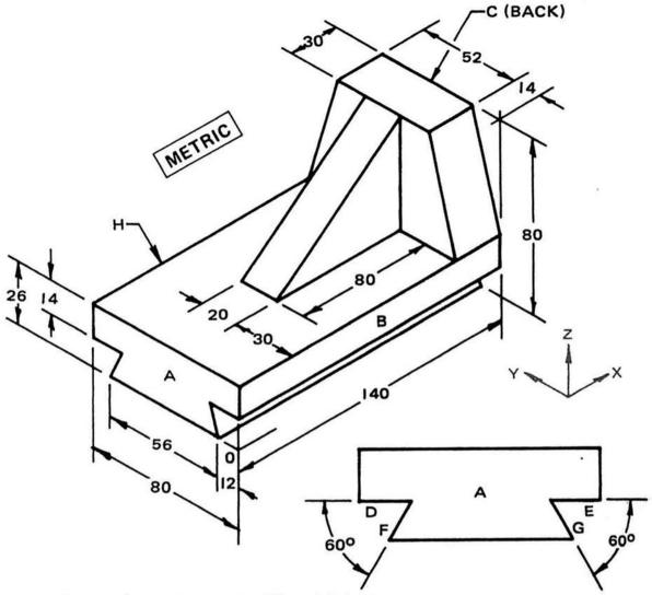
From the information shown in Fig. 16-218 make a three-view drawing of the cutoff stop.
